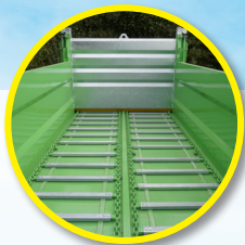
Double moving floor with bolted slats and shipping chains grade 80
