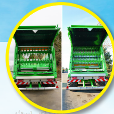
2 or 3 horizontal beaters with spreading table (2 x ø 1,040 mm)
